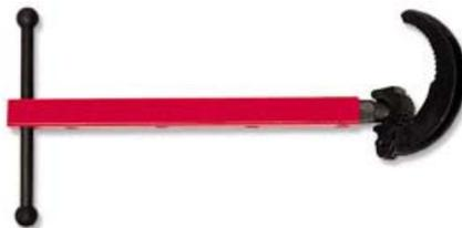
Basin wrench with 4-position telescopic handle for nuts and connections on washbasins, bathtubs, sinks or bidets. Min length: 280 mm, - L1: 340 mm, - L2: 400 mm, - L3: 460 mm. 180° pivoting fixed and moving jaw assembly mounted on the end of the handle. Return spring holds the jaw in place.
